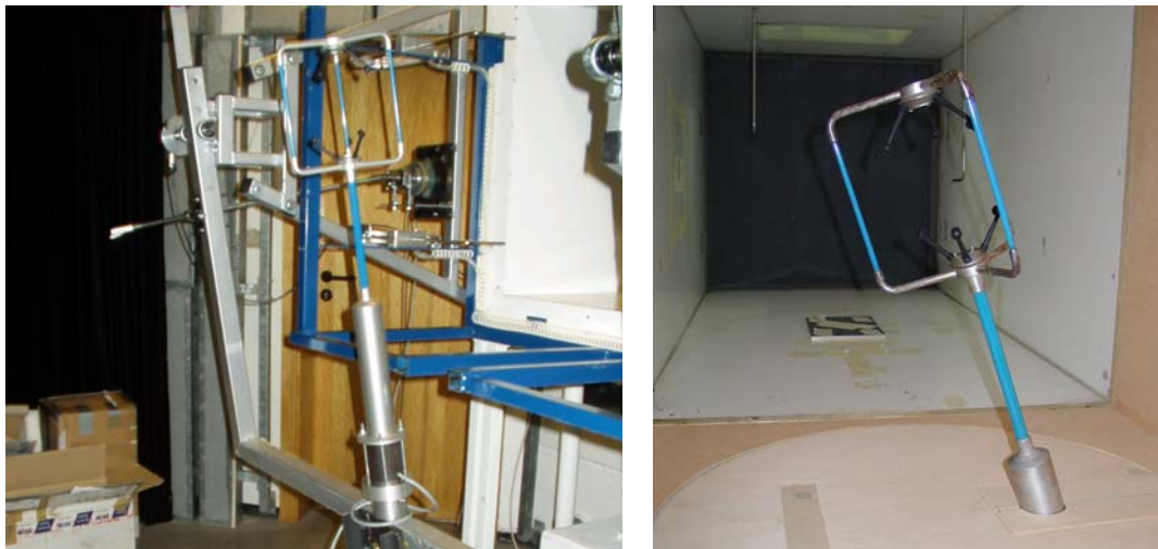
Figure 4-6 Gill Wind Master sonic during calibration at DEWI wind tunnel with tilting mechanism (left) and at IDR wind tunnel with tilted mounting on turn table (right), both methods keeping sensor centre at same position in wind tunnel during calibrations
