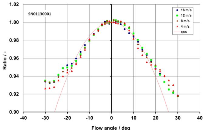
Five anemometers have been tested. Each individual tilt
