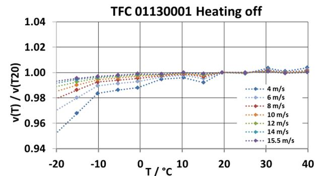
Five anemometers have been tested. Each individual temperature-ratio data have been used for classification
