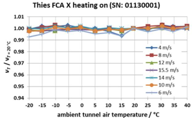
Five anemometers have been tested. Each individual temperature-ratio data have been used for classification
