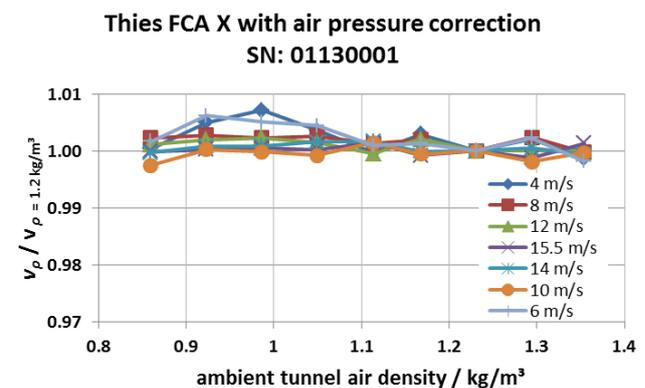
Five anemometers have been tested. Each individual air density-ratio data have been used for classification
